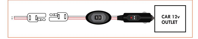
First connect the butt connector from the RV Waste Pump to the power wires of choice. Then find a suitable 12VDC Power Source and connect it.
