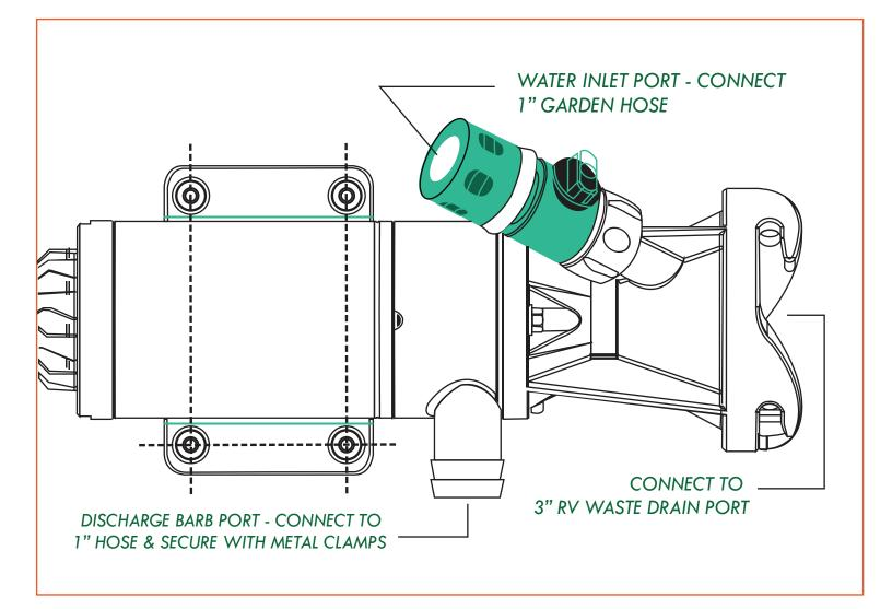
The LATCH.IT RV waste pump is the best solution for people always on the go. Empty out your holding tanks and avoid dumping stations. The macerator section of the LATCH.IT pump grinds down waste to a particle size of 1/8" so it can easily be pumped through a garden hose. Empty your holding tanks at a speed of 12.7 GPM!
